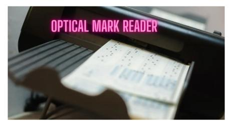
The laser light emits fewer amounts of light when the option is filled with black color; on the other hand, it reflects or emits less amount of light when there is no color.
